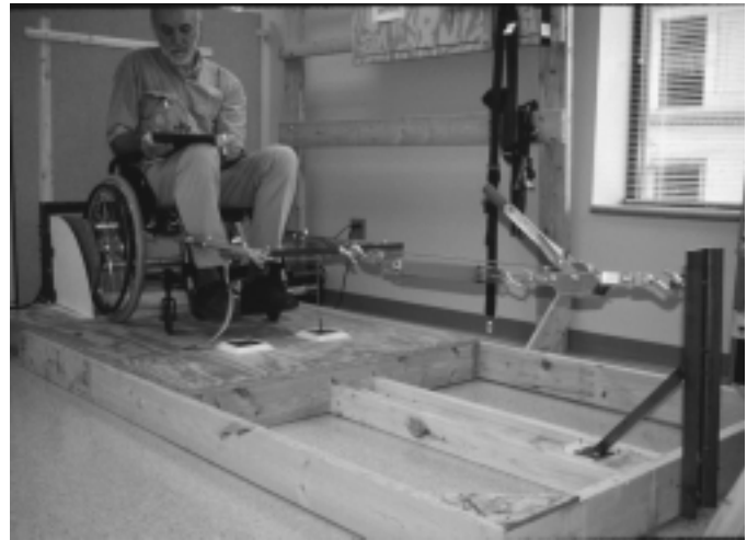
Figure 51 – Pull testing set up of the low “g” prototype securement device
