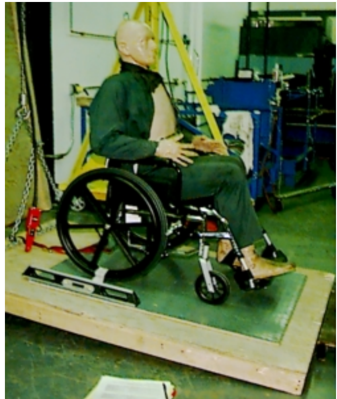
Figure 54 - Sliding test procedure using tilt platform
