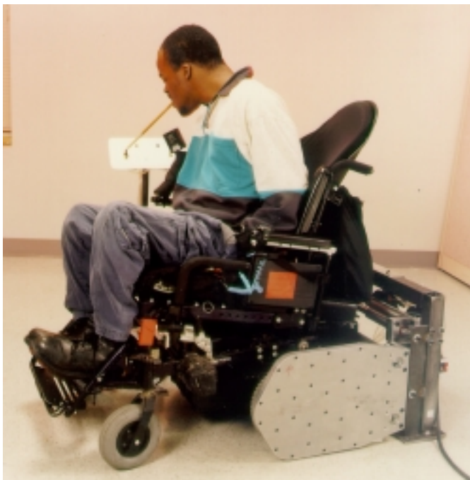
Figure 50 – Low “g” Docking System Securing Power Wheelchair
